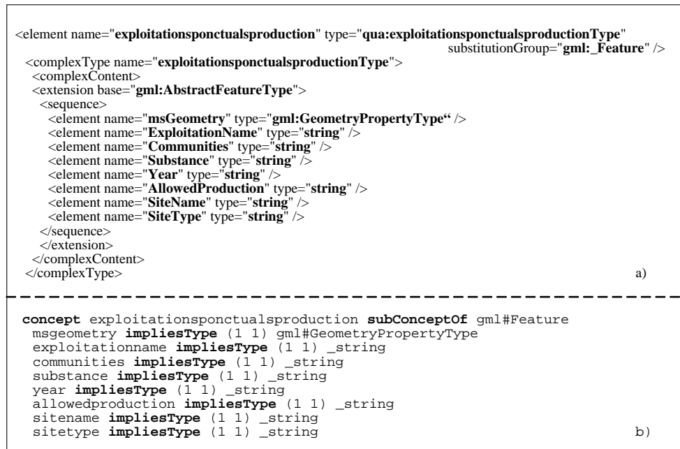
Figure 4: Transforming the feature type schema (a) into the FTO written in WSML (b).
