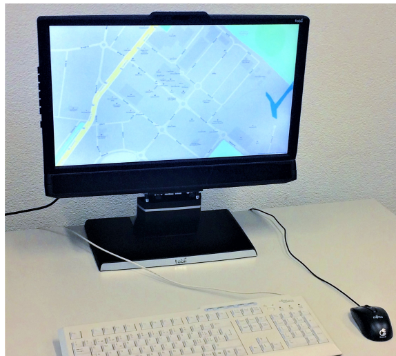
Figure 1: Setup for an eye tracking study on an online vector map with the FeaturEyeTrack framework.
