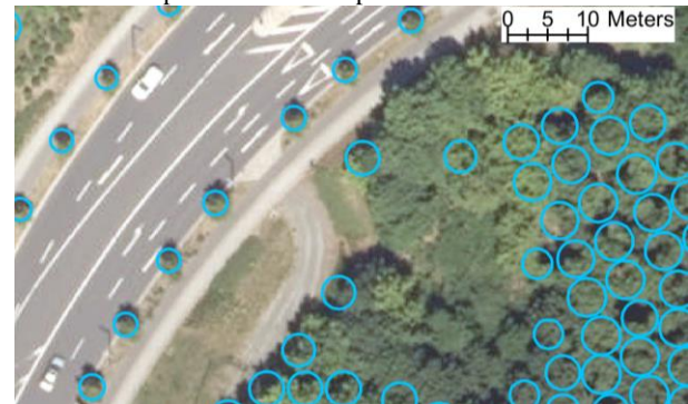
Figure 7: Predicted tree locations resulting from application of CNN1 with input formats 24x24 pixels (blue), 50x50 pixels (green) and 100x100 pixels (red)
